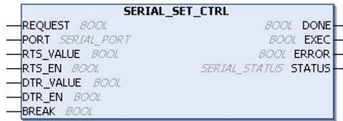
Figure 141: Block for Control Signals Writing
