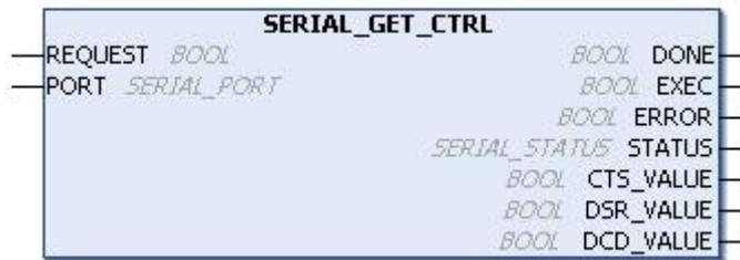
Figure 136: Block Used to Visualize the Control Signals
