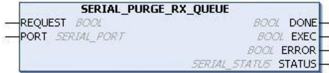
Figure 138: Block Used to Clean the RX Queue
