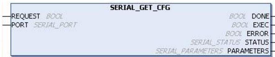
Figure 135: Block to Capture the Serial Configuration
