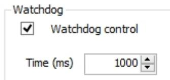
Figure 181: Watchdog Configuration of a PROFIBUS Remote
