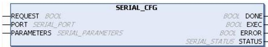
Figure 134: Serial Configuration Block
