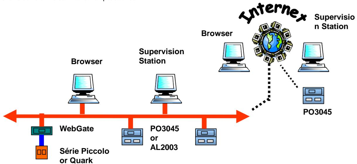
As shown on the diagram, all Altus controllers may now communicate through TCP/IP networks. Through the WebGate, old and brand new controllers from AL-600, Quark, Piccolo and AL-2003 Series also may take advantage of the Internet.
