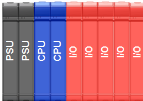
Figure 10: CPU Redundancy and Power Supply Module
