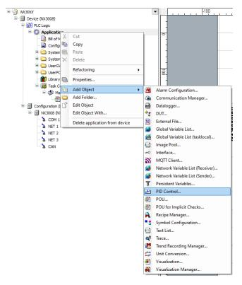
Figure 279: Steps to inserting the PID Control object in an application
