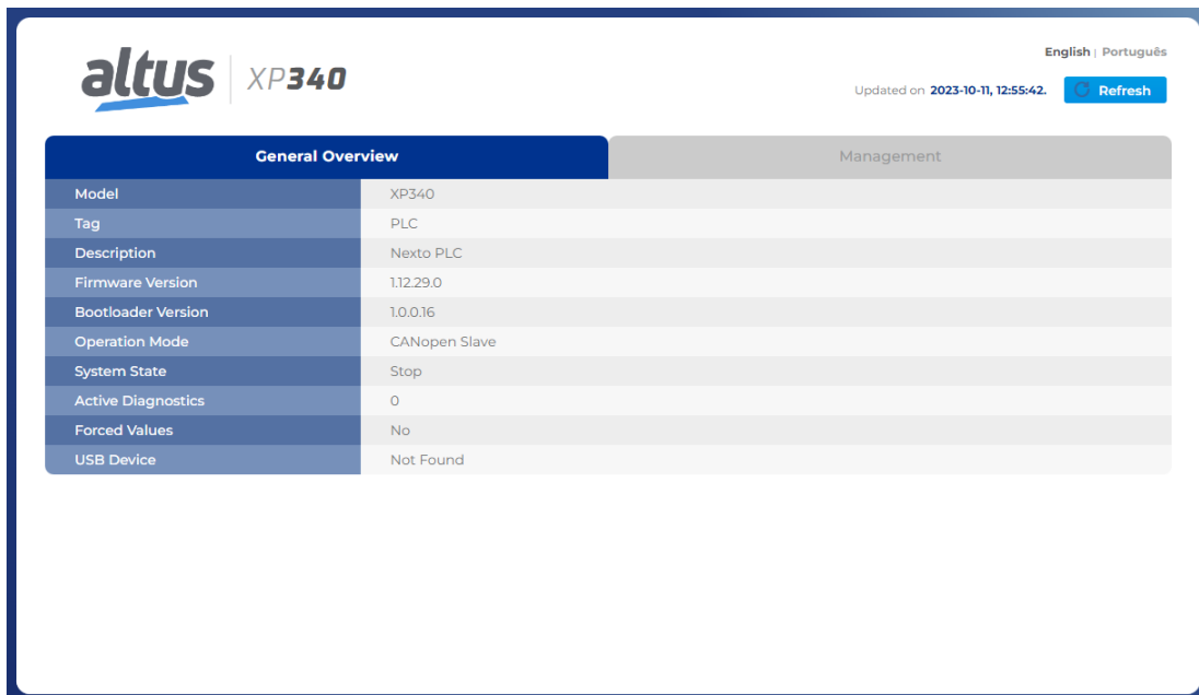
Figure 149: Operation Mode in the PLC Overview Screen
