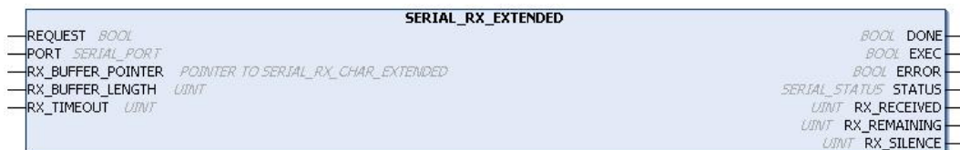
Figure 168: Block Used for Reception Buffer Reading
