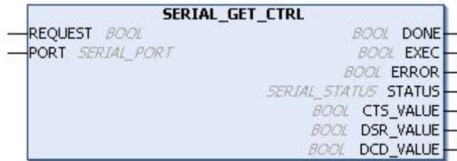
Figure 164: Block Used to Visualize the Control Signals
