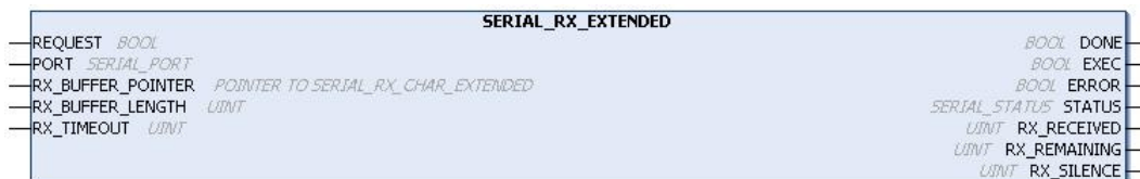
Figure 168: Block Used for Reception Buffer Reading
